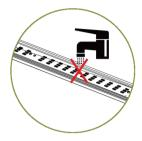
3. Please do not flush the LED surface to prevent damaging of LEDs.
