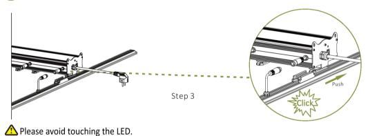
4.1 Connect the male plug of light bar to female plug of the driver box
