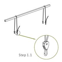
1.2 Pull the rope to adjust the fixture up; or press the lock to release or lower the fixture
