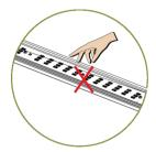
1.Please do not press the surface of LEDs to avoid damaging when installing the luminaire
