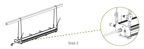
Push the light bar into the plastic buckle in the direction of the arrowhead until the buckle has a slight voice
